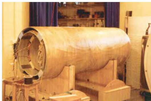
Figure 2. A doubly screened active magnetic shielded gradient coil for insertion in the superconductive magnet of Figure 1.
