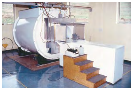
Figure 1. A home-built magnetic resonance imager with a 0.5 T super-conductive magnet.
